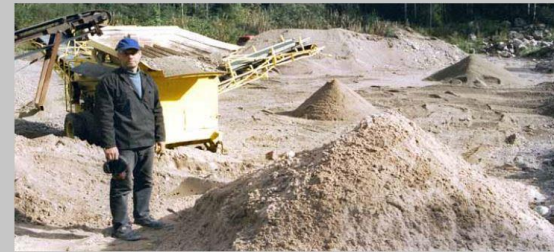
Kari Helenius stands beside a pile of crushed, screened sand in Teräskivi. To find a suitable aggregate can be laborious. Often, sands with different grain sizes have to be mixed to give the desired aggregate distribution. Ideally, ready-proportioned factory-made sand mixtures would be available in which the finest aggregate (grain size less than 0.075 mm) has been screened by laser or wind sieve.
